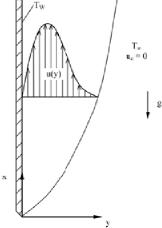
Free convection flow along a vertical flat plate. The flow and heat transfer for this case can be obtained from a similarity solution of the boundary layer equations and the energy equation.
