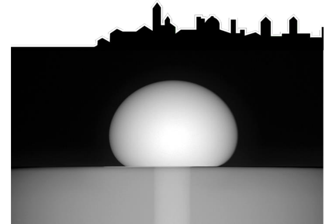
X-ray visualization of a liquid droplet growing from a single pore
